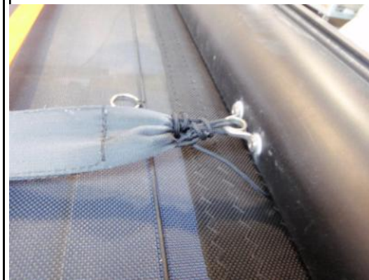
Spinnaker retrieve block Step 1 Go under the foot strap!
