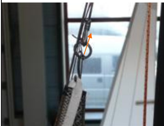
Step 2 and 3 Pull the jib up a bit and then twist the S hook with the halyard. Then pull the jib down.
