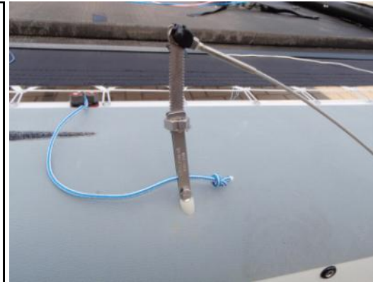
Fixing the stays and trapeze wires Step 1 Maximize staymaster length
