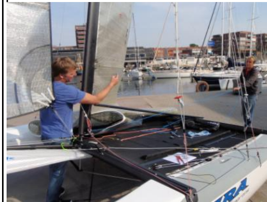
Step 3 Make sure the mast and the sail are facing the same direction while locking!
